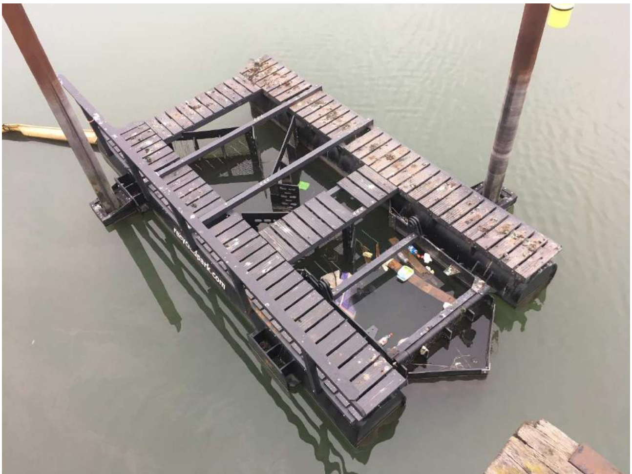
Figure 10. Waste collection device with waste guiding boom at left hand side, at the Port of Rotterdam, the Netherlands (Photo: M. Mannaart)
