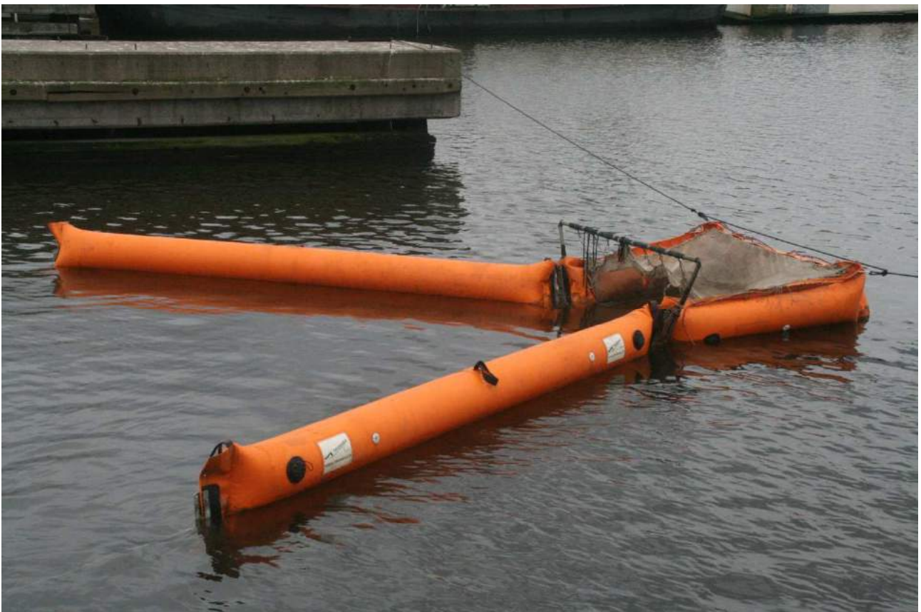
Figure 6: Floating litter collection device, applied to collect litter floating in the North Sea channel before drifting to sea, Part of a litter monitoring programme, the Netherlands (photo: M. Mannaart).
