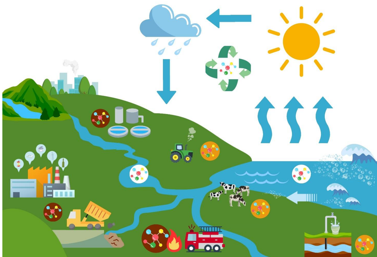
Figure 4. A simplified figure of the PFAS cycle with a focus on the marine environment. Sources are represented by dark red circles, transport routes with white circles, and potentially contaminated areas with orange circles.
